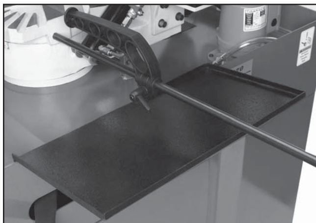
Figure 20. Splash tray installation.
